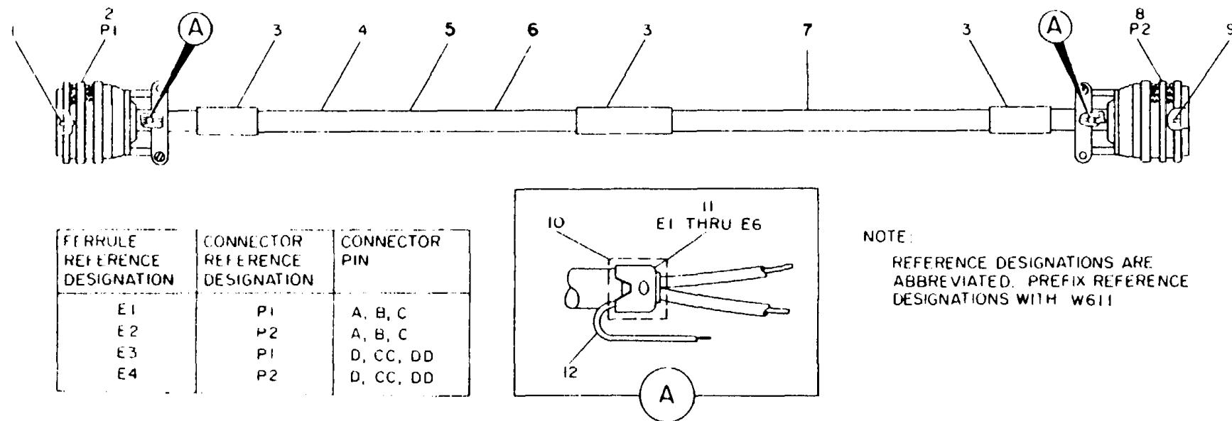
FIGURE 11. CABLE ASSEMBLY W611
