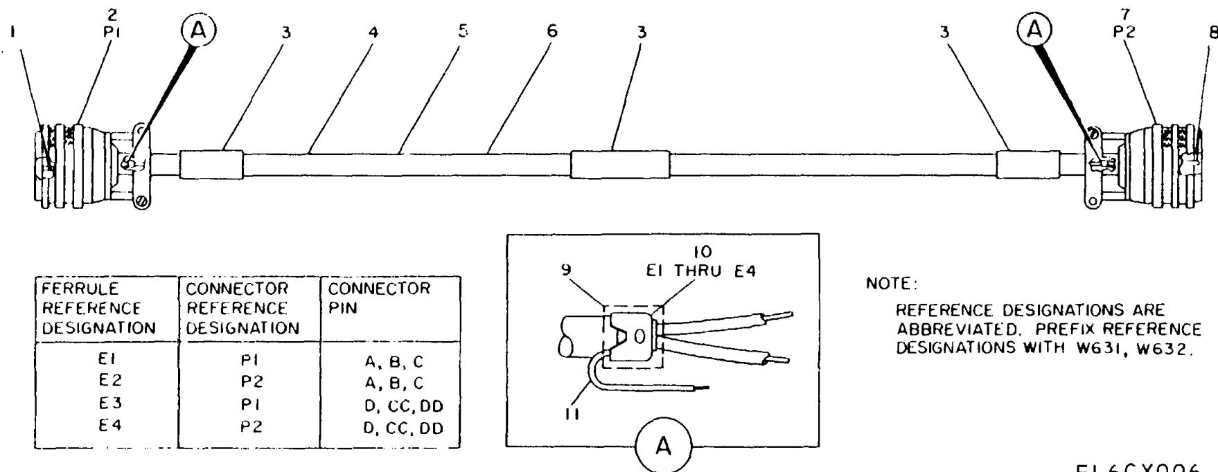
FIGURE 6. CABLE ASSEMBLY, W631
