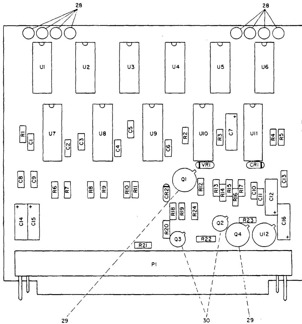
FIGURE 2. BUFFER COUNTDOWN CIRCUIT CARD 1A1
